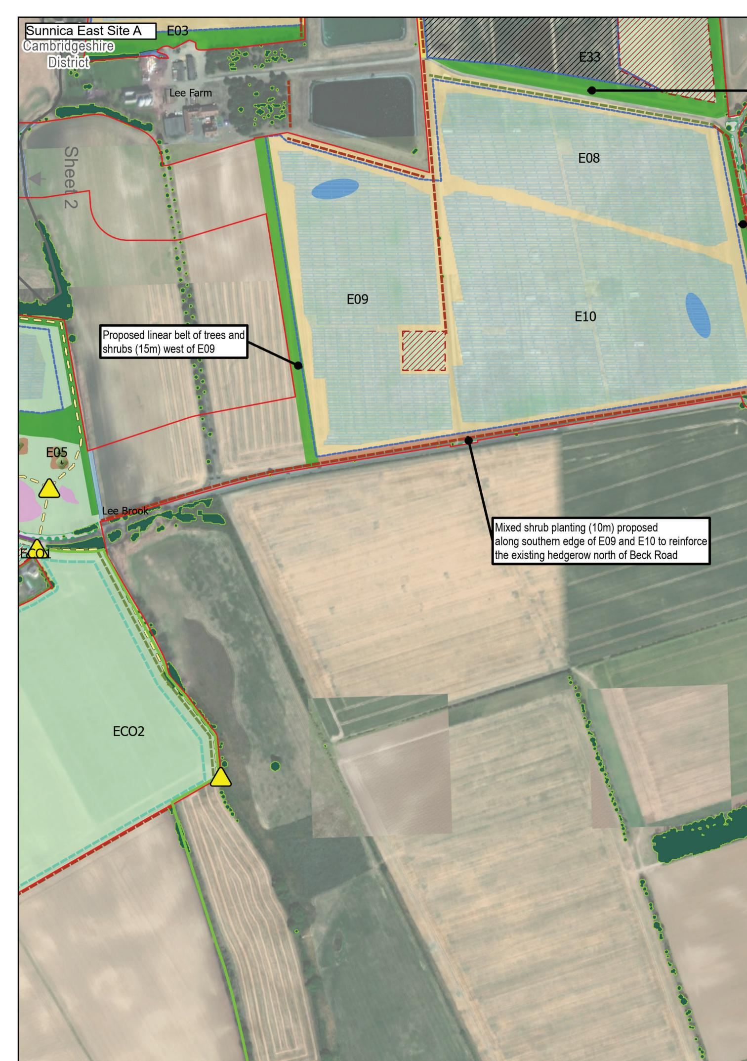
Linear belt of trees and shrubs (15m) and hedgerow planting to strengthen existing vegetation patterns, to enclose the BESS and substation and enhance habitat connectivity.
